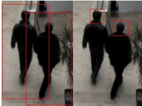
Figure 1: Example results after applying the HOG detector for pedestrians (left) and heads (right)
