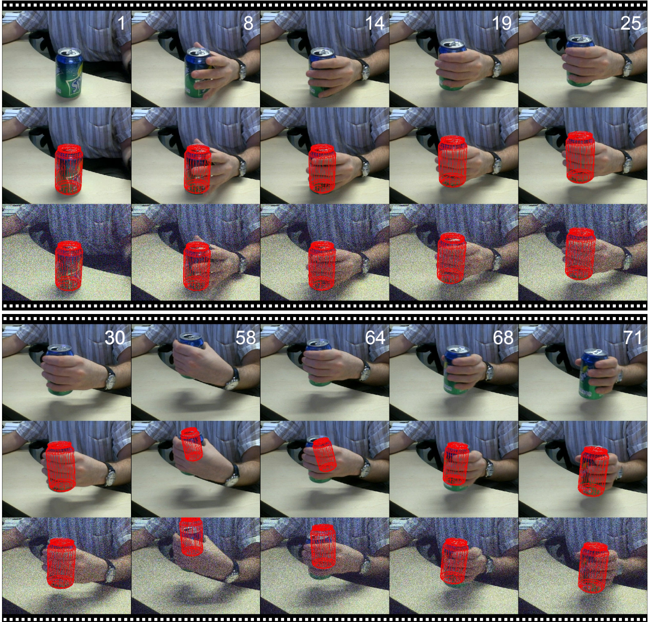
Figure 14: Film strip consisting of 10 frames from a video which showcases the PWP3D behaviour when subjected to occlusions and high levels of noise. For the first 6 frames (when both the top and bottom parts of the soft-drink can are visible) the pose is correct, even though most of the interior part of the object is occluded. When the bottom part of the can becomes occluded the pose becomes incorrect. The object moves “up” in the image because there is no longer a reason for it to stay “down”. The algorithm converges back to the correct position once the bottom part stops being occluded.
