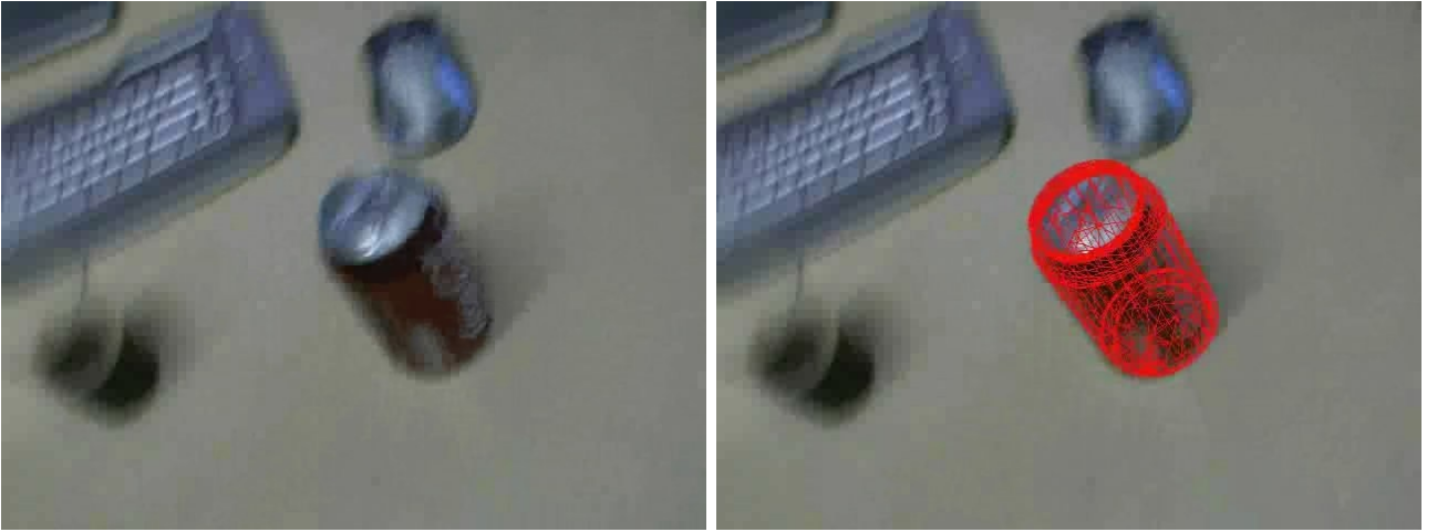
Figure 9: Robustness to motion blur. Left – original image, Right – recovered position.
