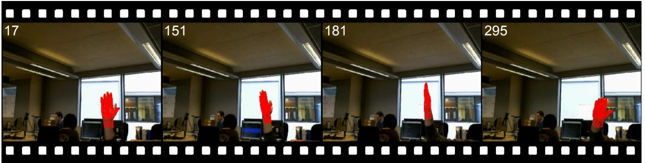
Figure 11: Film strip showing our method tracking a hand. Our algorithm can track the hand in this sequence at around 20fps.
