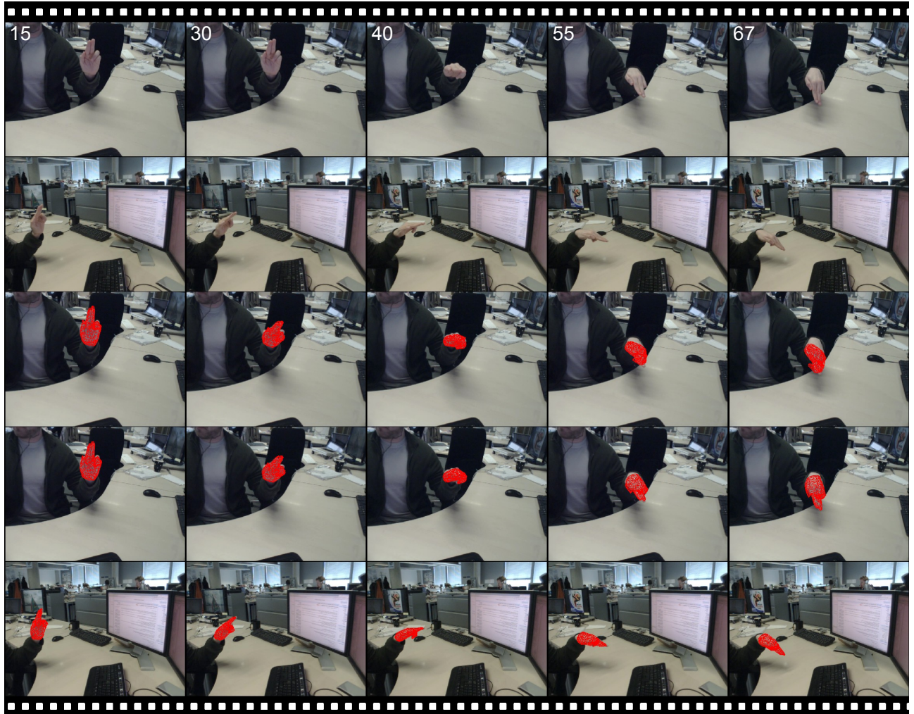
Figure 18: Multi view tracking. The top two rows show the two views. When processing only the first view (top row) the results are incorrect (third row) because the silhouette to pose mapping is ambiguous (multiple silhouettes can be generated by the same pose). When using two views the ambiguities are eliminated and the results are correct for both views (bottom two rows).
