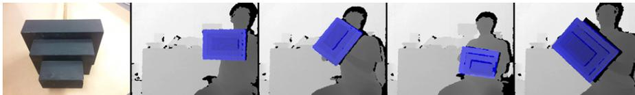
**Fig. 5.** The leftmost images shows our calibration object, Film strips to the right shows an example sequence that we used for simultaneous calibration and tracking.
